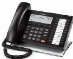
4-line Backlit LCD with 20 programmable buttons
